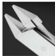
Squared beaks, clasp and wire bending plier, TC inserts.
